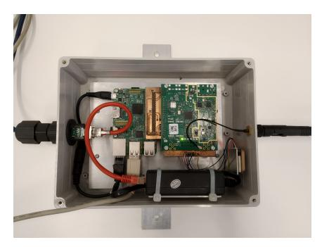
Figure 3.1: Gateway: Raspberry Pi 3 with IMST iC880A-SPI-LoRaWAN concentrator
